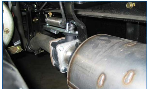
**NOTE: When routing the hoses care must be taken to keep hoses a minimum of 8" from the exhaust system.**
