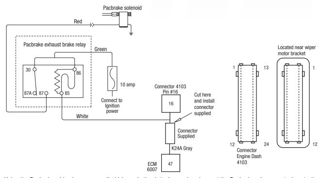
Using the Pacbrake wiring harness supplied (shown in the dotted area above) mount the Pacbrake relay receptacle onto the firewall using the self tapping screw provided. Install the relay.
