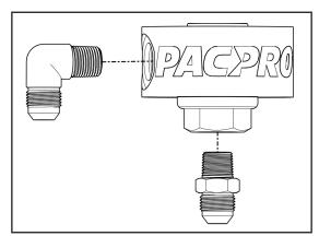
Install both seals onto the replacement filter head assembly as shown in figure 3. Put a light coat of clean engine oil on both seals and loosely install the assembly into the engine by turning the filter head retaining nut.
