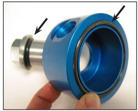
4 Rotate the replacement filter head assembly to attain maximum clearance for hose routing. Tighten the filter head retaining nut as you would for a new filter installation.
