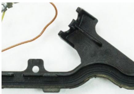
19B: Original Injector Harness Gasket
