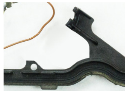
19D: Finished Modified Gasket
