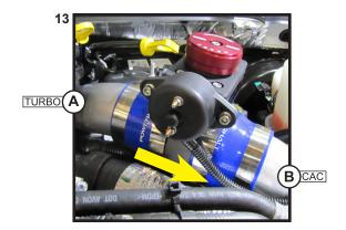
Place the second 3.5" clamp over the silicone reducer on the intercooler side of the CAC pipe.
