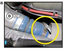
Rotate the pipe and the PowerHalt valve into position so that they are not rubbing or touching any other engine components. The reset knob should be somewhat horizontal with the top of the engine.
