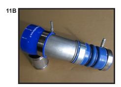
Attach the turbo side of the pipe onto the turbo outlet first. Push it on hard enough that the retainer clips into place.
