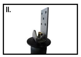
III. Loosely attached the lower bracket to the bottom of the air spring using a  $\frac{1}{2}$ " flat washer and  $\frac{1}{2}$ " -13 x  $\frac{7}{8}$ " hex head cap screw.
