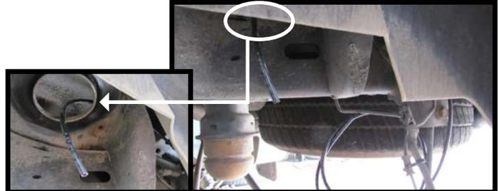
**NOTE:** Using scissors or wire cutters to cut the nylon airline WILL distort the line and cause the connection to leak. THE AIRLINE MUST BE CUT OFF SQUARELY WITH A SHARP RAZOR KNIFE. Moisten the end of the airline prior to inserting it onto the barbed fitting and push until it bottoms out.
