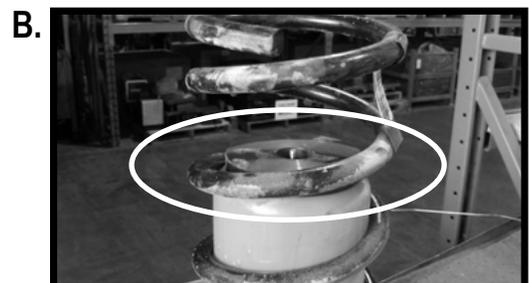
Insert the nylon spacer at the top (see photo B).
