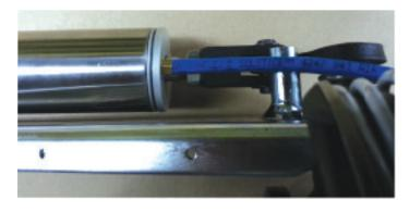
**Step 4** | Route the remote breather end of the hose to a clean dry area such as the engine compartment. Secure the hose using the supplied tie straps, away from heat sources and moving parts.
