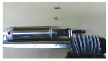
**Step 2** | Install the barbed fitting in to the cylinder vent port and torque to 15 in-lbs. Over torqueing WILL result in breaking the fitting in the threads.
