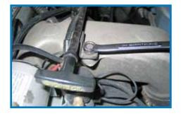
Disconnect the weather-pac electrical connectors to the compressor. Remove the three capscrews that hold down the compressor. Retain the spacers under the compressor bracket as they will be reused.
