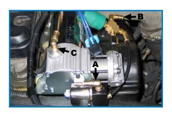
11 Consult with the customer for a preferred location for the quick connect airline coupler. Route the supplied airline to this location and connect to the coupler. Connect the other end to the remaining fitting at the compressor head.
