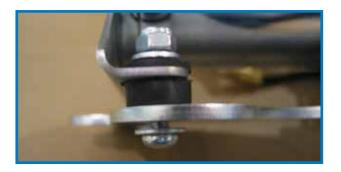
Position the correct length spacers in the locations shown in the photo (with arrows). All installations require the small O.D. spacer on the air intake horn.
