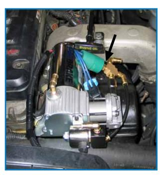
NOTE: The blind threaded port on the compressor head facing the front of the vehicle remains open.
