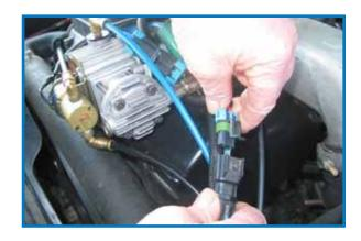
Connect the airline that is routed to the exhaust brake to the open fitting on the solenoid (labeled "A"). Connect the airline running to the air tank to either of the open fittings on the compressor head (labeled "B").
