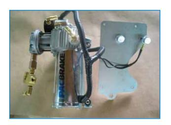
Tighten the four mounting screws and nuts until the washers first contact the isolator and then tighten TWO additional turns. Do not over tighten.
