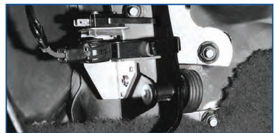
Connect the two red wires of the Pacbrake harness to the terminals shown above.
