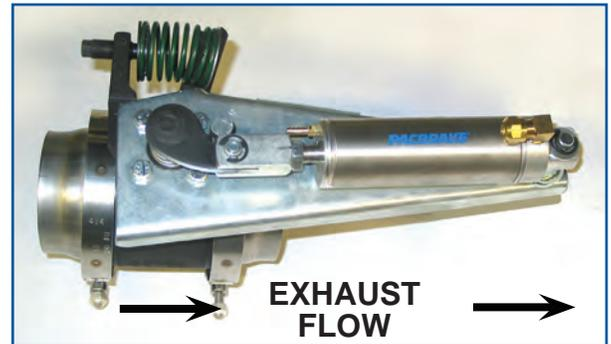
Note: any clamped exhaust connections between the brake and the engine must be welded at this time to ensure the joint can not separate or leak under pressure
