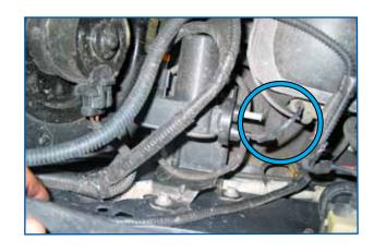
Remove the vacuum pump from the factory bracket, leaving the rubber isolators attached to the vacuum pump. Install the vacuum pump on to the Pacbrake supplied bracket as show in photo.
