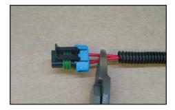
6 Connect the weather-pac connector of the new supplied harness to the new pressure switch. Route the other end of the harness to the drivers side battery and locate the black 16 awg. (ground) wire of the existing pacbrake harness. Cut this wire approximately 2" from the negative post of the battery. Strip ¼" off each end and crimp on the remaining two butt connectors. Shorten the new harness to the correct length if needed. Strip ¼" off each wire and crimp onto the butt connectors.
