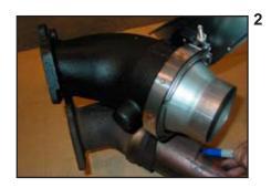
At the turbo charger check the gasket surface for imperfections. If okay, install the new gasket and replacement elbow provided. Replace the 5 capscrews removed earlier with the supplied 12 point fasteners. Torque the capscrews to 110 in-lbs in a star pattern, then re-torque to 220 in-lbs in a star pattern. After a road test, re-torque to all 5 capscrews 220 in-lbs.
