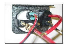
11 Connect the length of black airline provided to the paddle switch port marked "SUP". Route the black and red nylon airlines through the firewall boot into the engine compartment. The black airline connects to the air compressor discharge port. Ensure the end of the airline is cut squarely with a sharp razor knife. The red airline is connected to both air springs using the second barbed TEE fitting provided.
