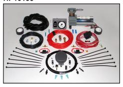
This kit contains "push to connect" airline fittings. They require the end of the airline inserted into the fitting to be round and cut clean/square to ensure the internal seal will not leak. The airline must only be cut with a sharp razor knife or sharp hose cutter. Using scissors or wire cutters will distort the end of the nylon tube causing the connection to leak air past the internal o-ring seal.
