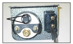
At the paddle switch, locate one of the two white wires. One wire needs to be connected to a good chassis ground. The remaining white wire of the paddle switch is connected to the white wire of the Pacbrake relay harness installed in step 8.
