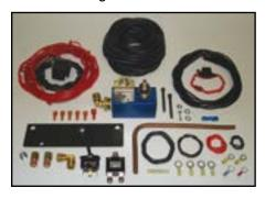
**NOTE:** This kit includes "push to connect" airline fittings. They require the end of the airline to be round, square and cleanly cut to ensure the internal seal will not leak air. The airline must only be cut with a sharp razor knife. Using scissors, a hose cutter, or wire cutters will distort the airline causing the connection to leak air past the o-ring seal.
