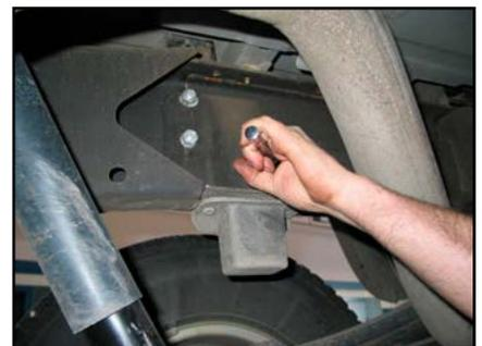
8 2500 models only (3/4 ton) may have a nut and bracket welded to the axle tube. It must be removed if interference exists with the lower air spring bracket.
