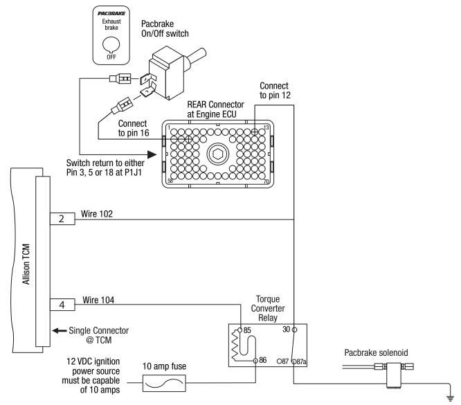
4th Generation Allison controls have the ability to be programed to communicate the downshift and torque converter unlock features over the Data-link J1939. Doing so eliminates the need to hard wire the exhaust brake circuit to the transmission ECU, the exhaust brake circuit only needs to be hard wired with the engine ECU. Consult your closest Caterpillar or Allison dealer for a quote, Pacbrake offers an interface kit C13074 if hard wiring is your preference.
