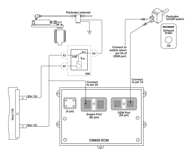
4th Generation Allison controls have the ability to be programmed to communicate the downshift and torque converter unlock features over the Data-link J1939. Doing so eliminates the need to hard wire the exhuast brake circuit to the transmission ECU, the exhaust brake circuit only needs to be hard wired with the engine ECU. Consult your closest Caterpillar or Allison dealer for a quote, Pacbrake offers an interface kit C13074 if hard wiring is your preference.
