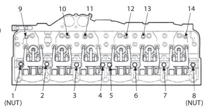
Jacob's model 790 utilized the J-lash® slave piston adjusting screw for lash adjustment. This model has a specific adjustment procedure therefore it must be adjusted as follows:
