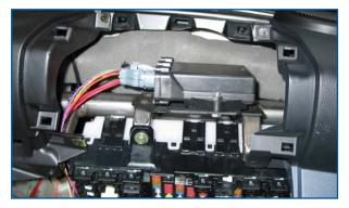
2 Above the fuse panel locate the three threaded holes in the fuse panel support bracket.
