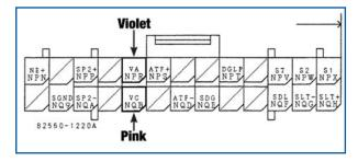
Connect the blue wire of the twisted pair to the violet wire of the transmission connector. Connect the red wire of the twisted pair to the pink wire of the
