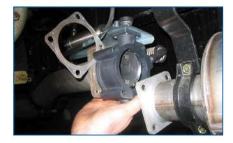
A length of nylon airline is supplied to connect the air cylinder to the solenoid. Connect one end of the nylon hose to the 90° fitting and route the other end to the engine compartment.
