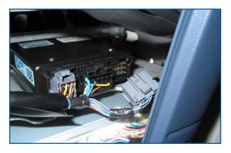
Feed all the unconnected wires through the firewall boot in the upper passengers side of the firewall into the engine compartment. Some model trucks have firewall grommet near the accelerator pedal under the floor mat that can be used.
