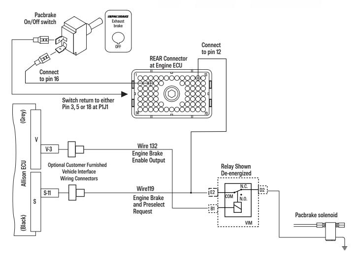
The switch input at J1/P1:16 requires that the "Exhaust Brake Switch" be programmed to "Installed". The Parameter "Exhaust Brake Warm-Up Configuration" must be programmed to "Exhaust Brake Only" or "Exhaust Brake & Warm-up".
