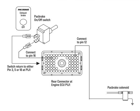
The switch input at J1/P1:16 requires that the "Exhaust Brake Switch" be programmed to "Installed". The parameter "Exhaust Brake Warm-up Configuration" must be programmed to "Exhaust Brake Only" or "Exhaust Brake & Warm Up".
