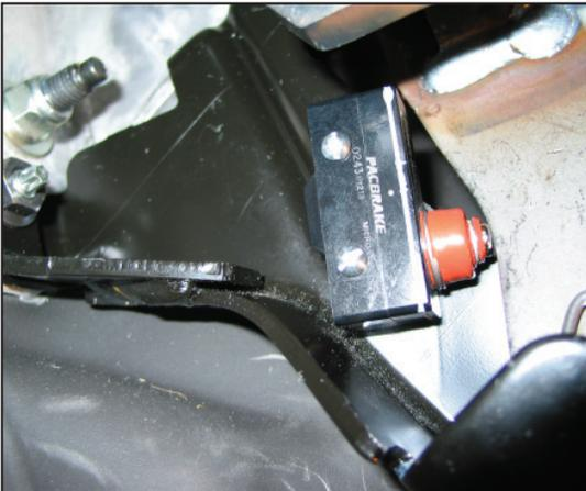
The engine's ECM has a built-in delay for exhaust brake application. This mechanical kit was developed to reduce the delay and speed up the application time of the exhaust brake. Pacbrake also offers an optional air tank kit (C11941) to speed up the application of the exhaust brake.
