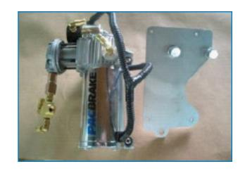
Machine screws must be installed as shown in the photo (threaded ends pointing upwards).
