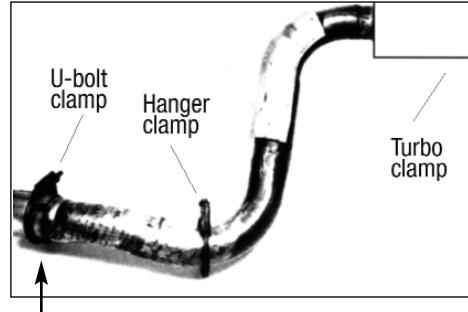
**NOTE: Some trimming may be necessary to provide close mating prior to installation of clamp.**
