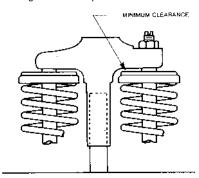
**CAUTION!** After cross-head installation and adjustment it is imperative that a clearance check is made between the underside of the cross-head on the adjusting screw side and the top of the valve rotocoil.
