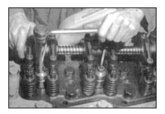
Remove the front rocker shaft group from the engine.
