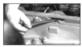
Install the solenoid wire on the spacer lead-out terminal.
